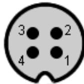
Figure 31: 4-pin circular plug-in connector (female)
