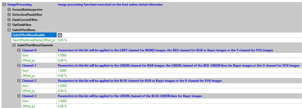
Figure 3: The configuration field for the GainOffsetKnee filter
